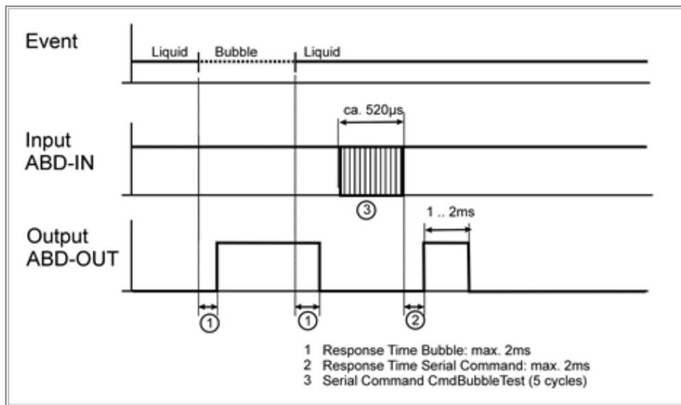
Figure 5: Signal on Output in Interface Mode 1
