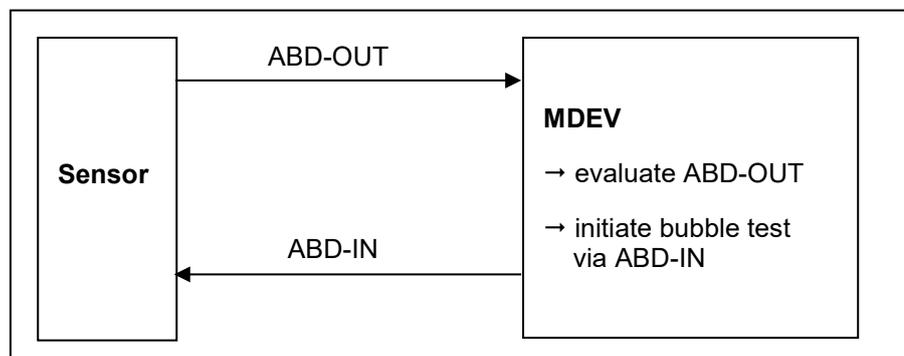
The sensor has no direct access to control components. All bubble detection results are transmitted to the machine via signal lines. An alarm handling must be implemented in the medical device.
