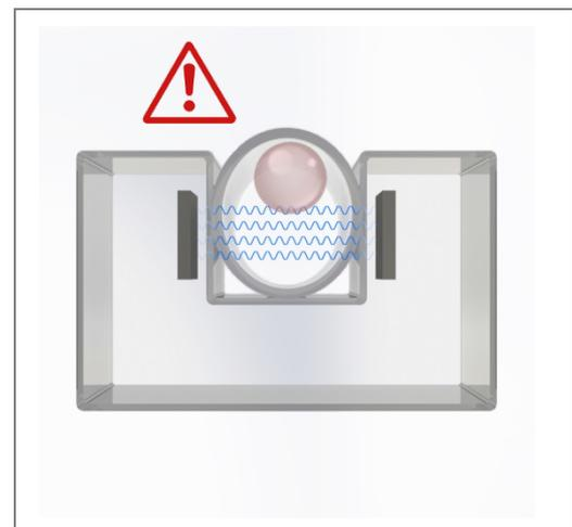
Figure 11: Poor bubble sensitivity due to sensor orientation [symbolic representation: not in scale, blue wavy lines = ultrasonic path]
