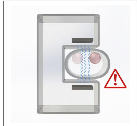
Figure 9 | 10: Tube too small / too large [symbolic representation: not in scale, blue wavy lines = ultrasonic path]
