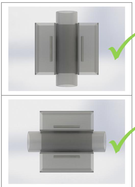
Figure 12 / 13: Good bubble sensitivity: vertical or horizontal position [side view]
