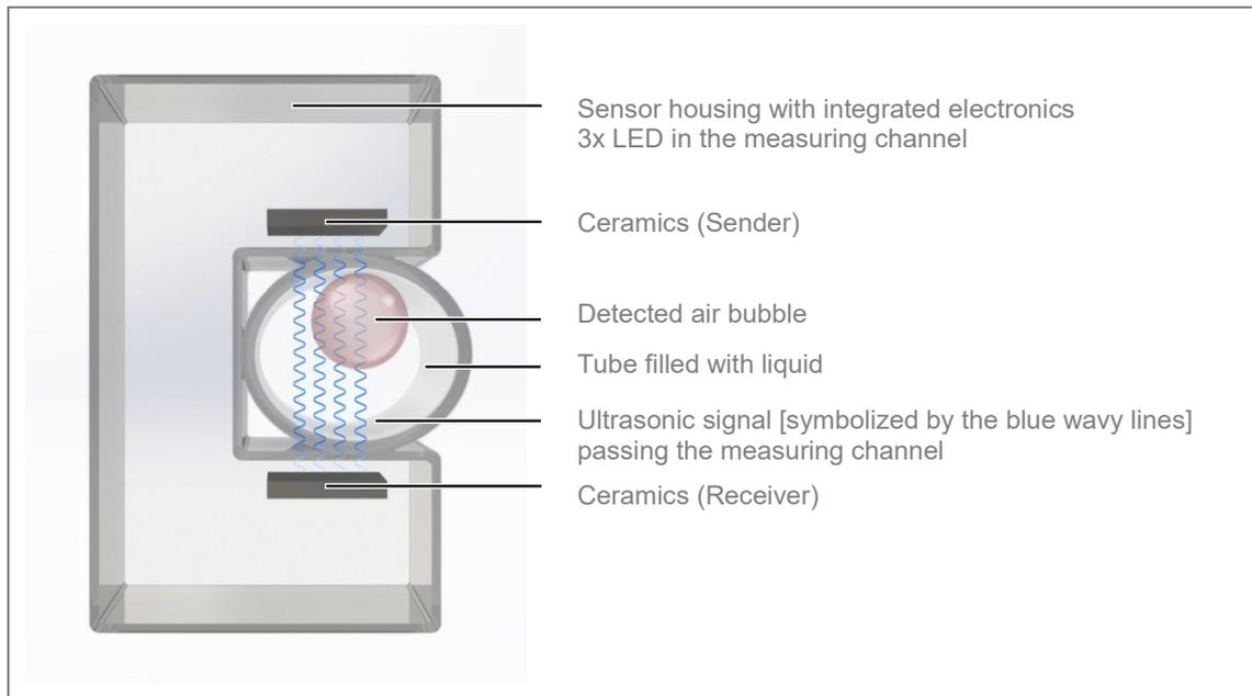
Figure 2: Sensor design and function [symbolic representation]
