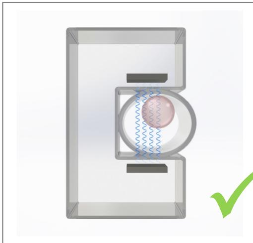
→ **Tubing fits in the measuring channel:** coupling surface is sufficiently large for the coupling of ultrasound, tube is not squeezed
