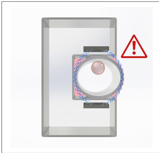
→ Ultrasound may be conducted past the tube to the receiver.
