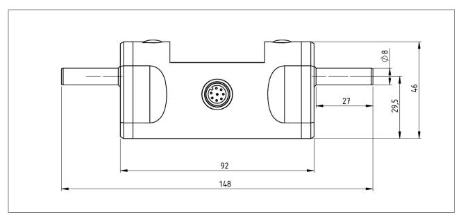
Figure 1: Dimensions SONOFLOW® IL.52/3 V2.0 - Side view
