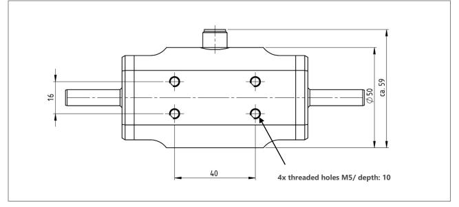
Figure 2: Rear side with drill holes for mounting
