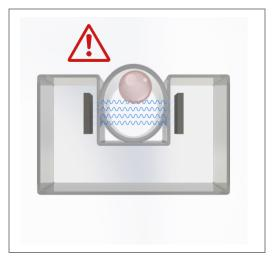
Figure 11: Poor bubble sensitivity due to sensor orientation [symbolic representation: not in scale, blue wavy lines = ultrasonic path]
