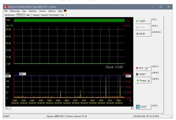
Figure 16: Screenshot of ABD Monitor - typical tracking of bubbles: Tiny bubble (no alarm) / small bubble (alarm is just released), for released alarm see the status bar
