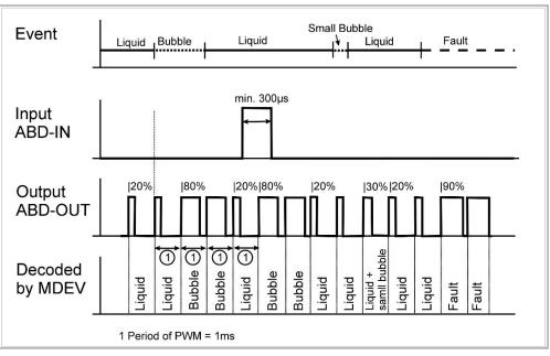
Figure 7: Signal on Output in Interface Mode 7
