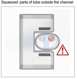
Figure 9 | 10: Tube too small / too large [symbolic representation: not in scale, blue wavy lines = ultrasonic path]
