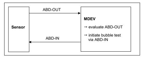
The sensor has no direct access to control components. All bubble detection results are transmitted to the machine via signal lines. An alarm handling must be implemented in the medical device.
