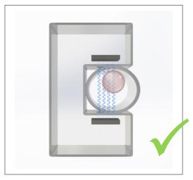
$\rightarrow$  **Tubing fits in the measuring channel:** coupling surface is sufficiently large for the coupling of ultrasound, tube is not squeezed
