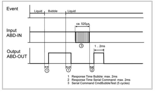
To check the sensor functionality, the serial command CmdBubbleTest can be used.
