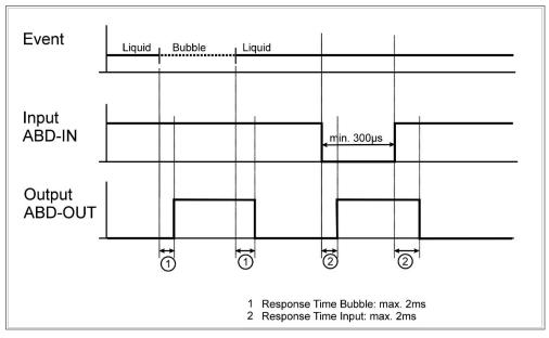
Figure 6: Signal on Output in Interface Mode 4
